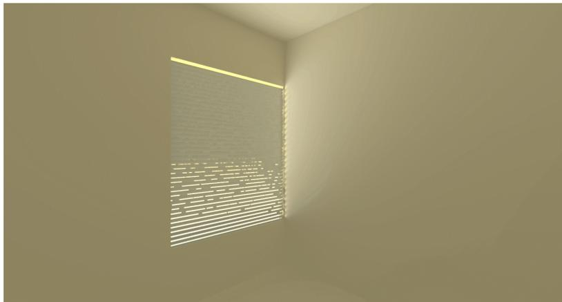
*Figure 3. Highlights on side wall are smaller when the window is subdivided vertically into three different window areas (see next Figure). Note: Blinds are at a different angle here than in the previous figure.*
