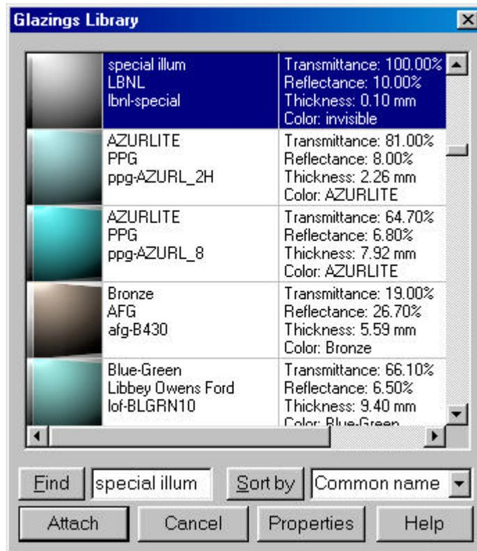
Figure 9 - The special illum glazing that is assigned to a surface that covers a window or skylight aperture to consider it as a light source.
