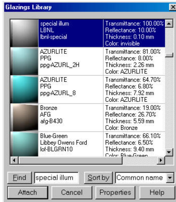
Figure 6. The special illum glazing material used with mkillum.
