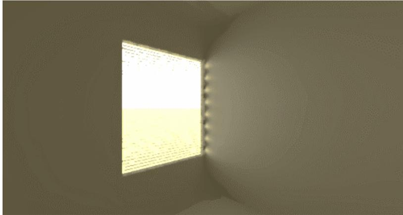
*Figure 4. Highlights on side wall with mkillum since window is only subdivided into a maximum of 8 pieces along any dimension.*
