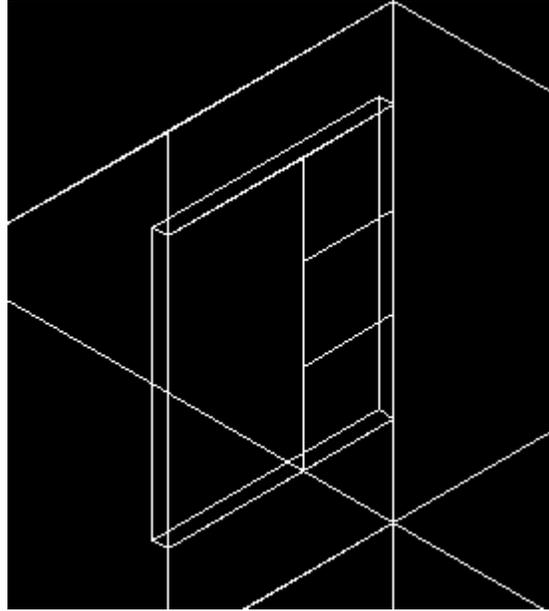
*Figure 5. The window in the previous figure has been divided into three different areas along the side wall to reduce the size of the highlights on the side wall. 24 window sources (instead of 8) will be applied along the right side of this window at a high accuracy setting.*
