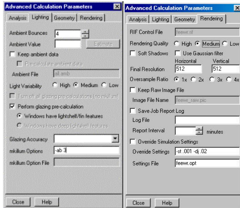
Figure 2. The number of ambient bounces can be set for both the interior and the mkillum calculations. Rendering quality and soft shadows (penumbras) can also be specified.
