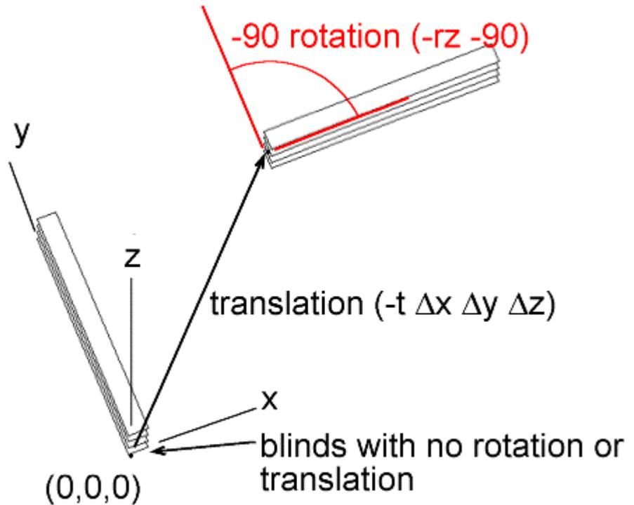
Figure 10 - Blinds that are not rotated or translated are aligned with the y-axis with a corner located at the origin (0,0,0). They must be rotated and translated place them at their appropriate room position.
